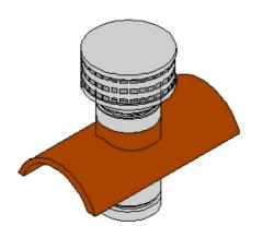
The Dunbrik Gastyle II ridge vent terminal is designed for use with domestic gas flue block systems using 127mm internal diameter twinwall flue pipe. The efficient design helps overcome difficult site conditions caused by prevailing winds and high-pressure zones.
