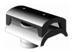
The Dunvent is a traditional low profile ridge vent terminal for use with domestic gas flue block systems using 127mm internal diameter twinwall flue pipe. It has a 127mm round flue pipe connection, avoiding the restrictions of a rectangular ridge tile adaptor. It fits to the ridge line and wire mesh keeps out birds and debris.
