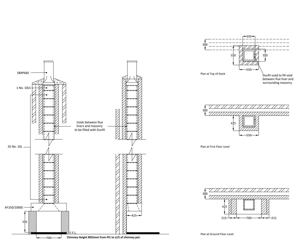
Dunbrik A1 Concrete Flue Liner System to BS EN 1857
