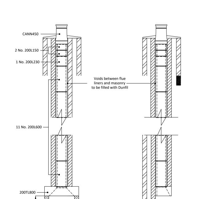
Chimney Height 8010mm from FFL to U/S of chimney pot.
